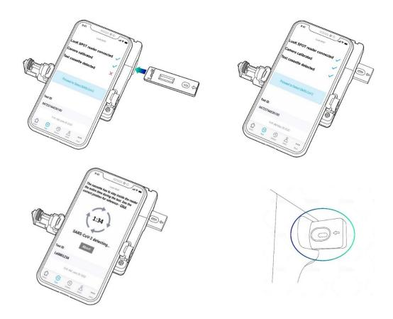
4. The test result will be ready between 5 to 8 minutes on the Look SPOT app screen. The results can be Positive, Negative, or Invalid. For an invalid test result, please proceed with the Calibration process and redo the test again because the phone may clean up the settings due to a long period of use.
