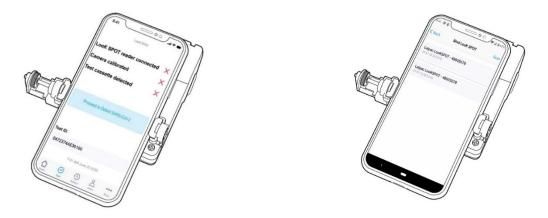
Once the Look SPOT is connected via Bluetooth with the smartphone, insert the calibration cassette. Then press the X mark of "Camera Calibrated" to calibrate the camera.
