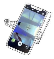
Open the Look SPOT app. Make sure the smartphone has Bluetooth enabled (For Android OS, please also enable the Location Service for the Bluetooth connectivity to work). Press the X mark of "Look SPOT connected" to see the available Look SPOT to connect. Select the correct Look SPOT based on the serial number on the sticker of the Look SPOT. Once selected, press Back.
