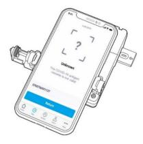
The test results are documented automatically in the History section of the Look SPOT app with the Test ID, location, city, country, and timestamp of the tests. If the test did not flow correctly, the test result would show Invalid. Shall the invalid test result occur, please repeat the Calibration process and initiate a new test with the same test cassette or a new test cassette with a new nasal swab sample.
