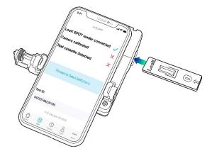
The screen will show the view of the calibration cassette and a small white box. Press the Calibrate button to calibrate. A message of Processing will appear. Wait until it is done. Then press Confirm.
